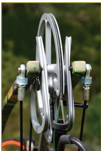
The distinctive cams on the Liberty I are widespread to better balance the entire bow and facilitate its shoot-through nature.
